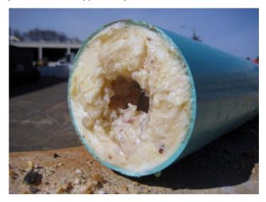
The problem is that oil and grease, when placed in facility drains, causes blockages and corrosion in downstream sewer pipes, requiring sewer pipes to be cleaned or replaced. To address this problem, the installation and maintenance of grease interceptors is required at restaurants, convenience stores and other food service facilities.
