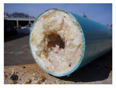
The problem is that oil and grease, when placed in facility drains, causes blockages and corrosion in downstream sewer pipes, requiring sewer pipes to be cleaned or replaced. To address this problem, the installation and maintenance of grease interceptors is required at restaurants, convenience stores and other food service facilities.
