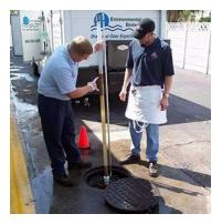
into the interceptor contents near the influent and effluent pipes and retrieve a sample. Measure and record the thickness of the grease and the solids layers. Use a sludge sampler, like the TruCore Sludge sampler (pictured), to measure the thickness of the layers.
